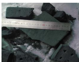
粉碎前 约200×160×t55mm Before crushing
