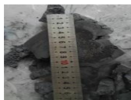
粉碎前 (约140 × 110 × t35mm) Before crushing
